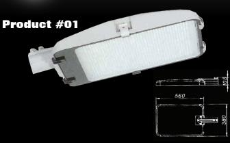
Power: 60W (35-110W) Luminouos Flux: 5100 Color Temperature: 2700-6400 Lux/Distance: 30/8 Scope: 25 Color Rendering Property: 70-80 Protection Glass: 65
